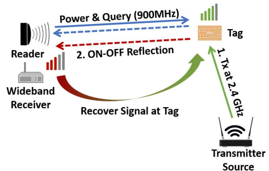
Figure 1: Commercial RFID tags powered by a 915 MHz RFID reader, also backscatter signals at other frequencies. RFIMap exploits this to recover the signal power incident at the tag at desired frequencies.
