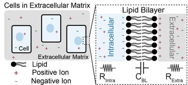
**Figure 2: The bio-impedance of tissues is a complex number that consists of a resistance (real) part contributed by the aqueous ions inside and outside cells, as well as a capacitance (imaginary) part contributed by the lipid membrane barriers.**
