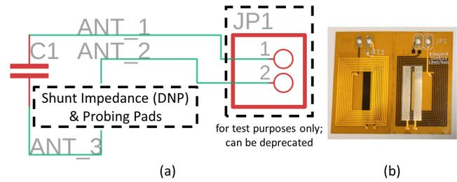
**Figure 8: The coils on a NFCapsule pill device has a simple circuit layout. The shunt impedance can be connected in parallel with the target tissue during actual tests. Meanwhile, the jumper is designed solely for test purposes.**
