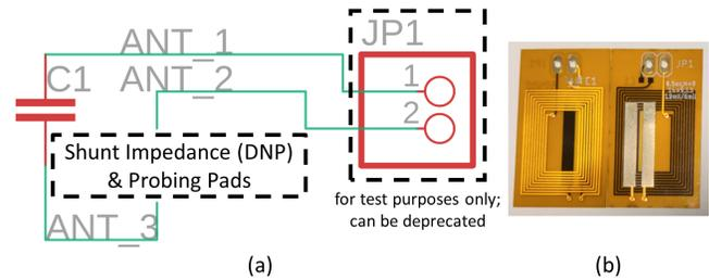
**Figure 8: The coils on a NFCapsule pill device has a simple circuit layout. The shunt impedance can be connected in parallel with the target tissue during actual tests. Meanwhile, the jumper is designed solely for test purposes.**
