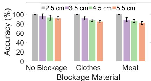
**Figure 13:** NFCapsule’s classification accuracy on gel models with blockage. The result is grouped by material on the X-axis; each group contains four accuracy values of different reading ranges. We see clothes and meat induce similar performance drop to NFCapsule.
