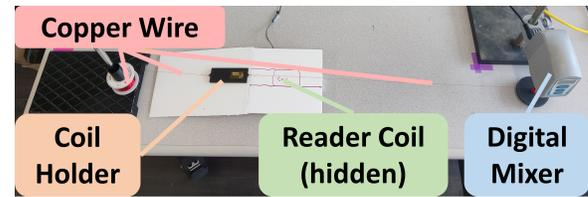
**Figure 15:** NFCapsule’s translation experiment setup. A digital mixer is used to wind the copper wire. The coil holder moves over the reader coil with a controlled and consistent speed to emulate the movement in a swallowing behavior.
