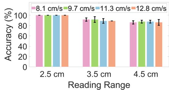
**Figure 16:** NFCapsule’s classification accuracy on gel models with different moving speeds. The result is grouped by reading range on the X-axis. Overall, a moving coil does not introduce much performance fluctuation.
