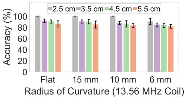
**Figure 14:** NFCapsule’s classification accuracy on gel models with varying radius of curvature. The result is grouped by radius on the X-axis; each group contains 4 accuracy values of different reading ranges. A smaller radius causes more performance drop; 6 mm is close to our capsule’s actual size.
