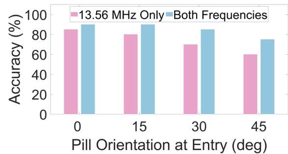
**Figure 18:** NFCapsule’s end-to-end performance with different pill orientations at entry. The result is grouped by pill orientation. We see that operating at both frequencies help NFCapsule better distinguish between healthy and damaged tissues; yet, a misalignment between the reader antennas and the coils on the pill introduces a performance drop.
