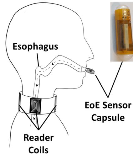
**Figure 1: NFCapsule includes a reader device worn at the user’s neck with multiple coil antennas (to be integrated into a flexible choker in the future) and an EoE sensor capsule that interacts with the user’s esophagus tissue.**
