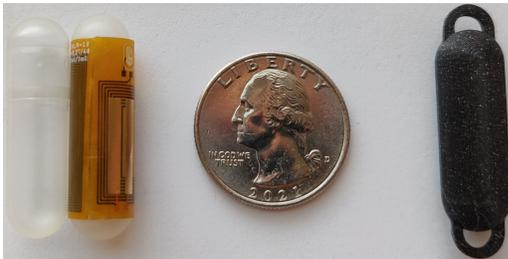
Figure 10: NFCapsule pill device prototype with a gelatin capsule (27 mm height and 10 mm diameter) and a 3D-printed capsule mold for movement tests.
