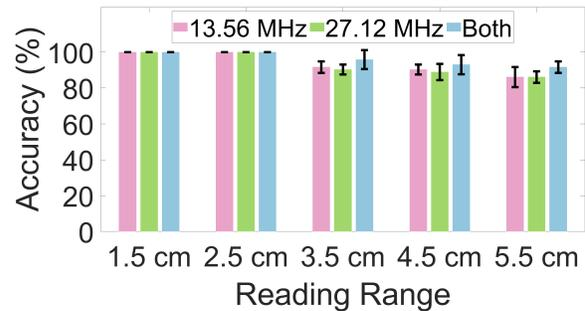
**Figure 12:** NFCapsule’s classification accuracy on gel models with both kinds of coils. The result is grouped by reading range on the X-axis. Overall, combining the collective information from both coils helps improve the accuracy.
