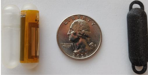
Figure 10: NFCapsule pill device prototype with a gelatin capsule (27 mm height and 10 mm diameter) and a 3D-printed capsule mold for movement tests.
