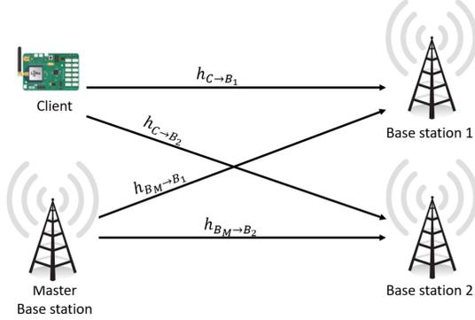
Figure 5: **Wireless channels** between client and base stations
