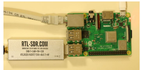
(c) CharIoT's gateway prototype- RTL-SDR+RPI.
